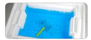
d. When the exposure time has elapsed, rinse the sensor thoroughly with water. Prevent jets of water from entering the sensor opening.
