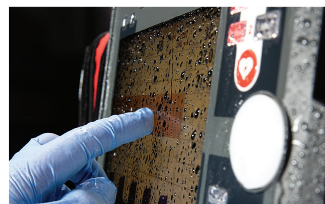
► TOUCH 'N DIAL on the C3T : Operation via JogDial or optionally via touch.
